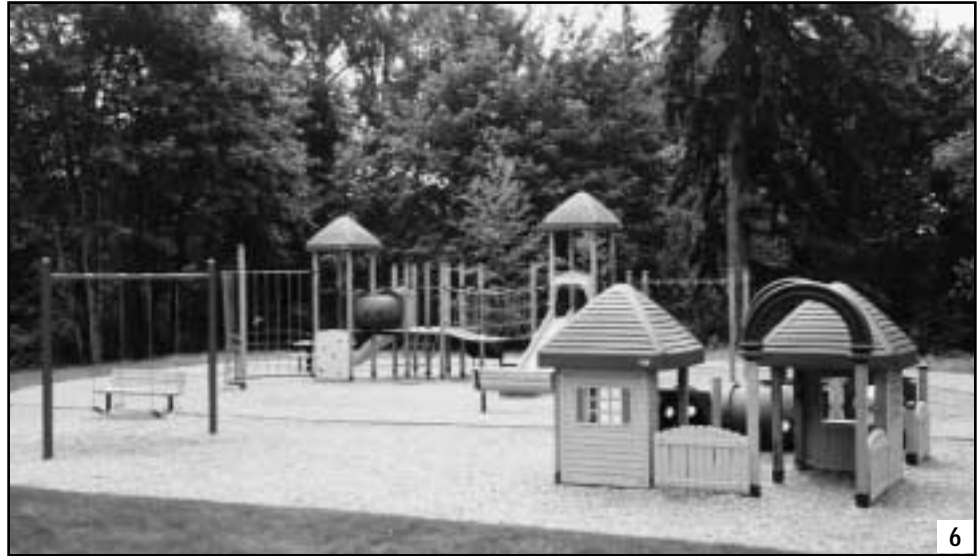
This dual play area designed for 2- to 5-year-olds and 5- to 12-year-olds shares resilient surfacing. Each section must be evaluated separately.
